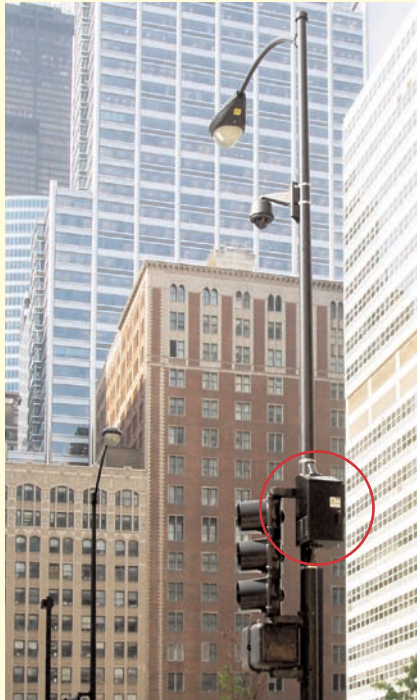
Custom enclosure, circled in red, with Firetide node inside
